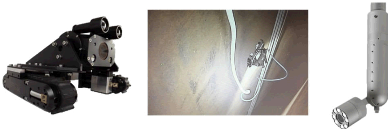
Figure 6-7. Pan-Tilt-Zoom and Magnetic Crawler Camera Hardware
