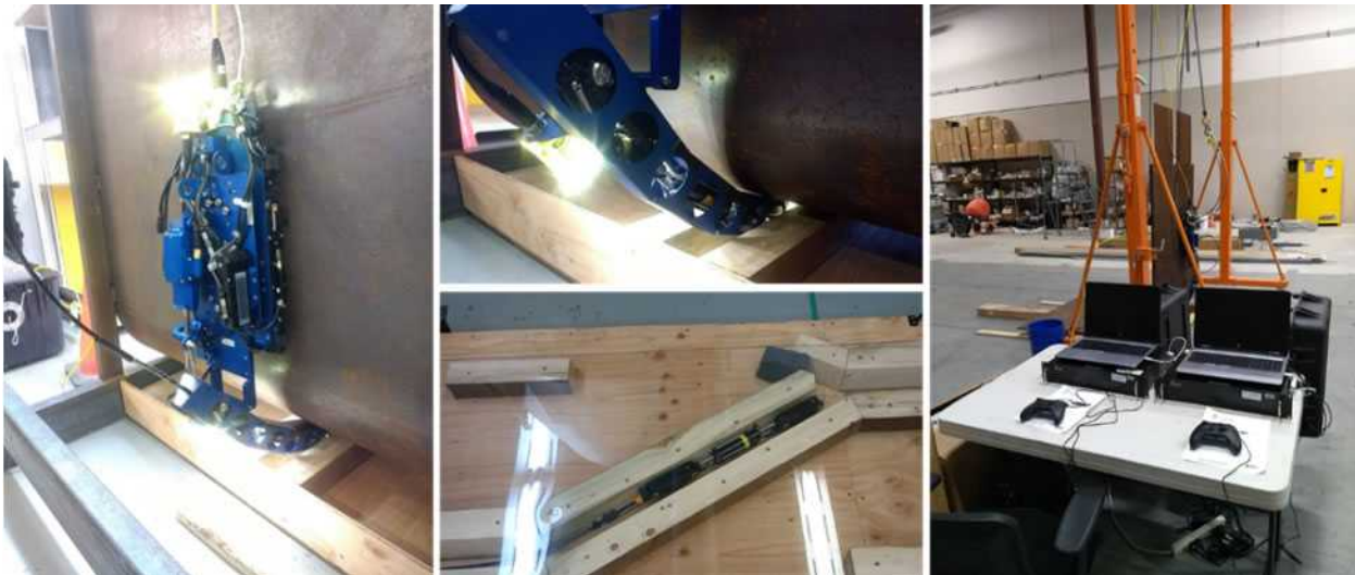
Figure 6-5. Fabricated Veolia/Inuktun Tank Bottom Inspection System
